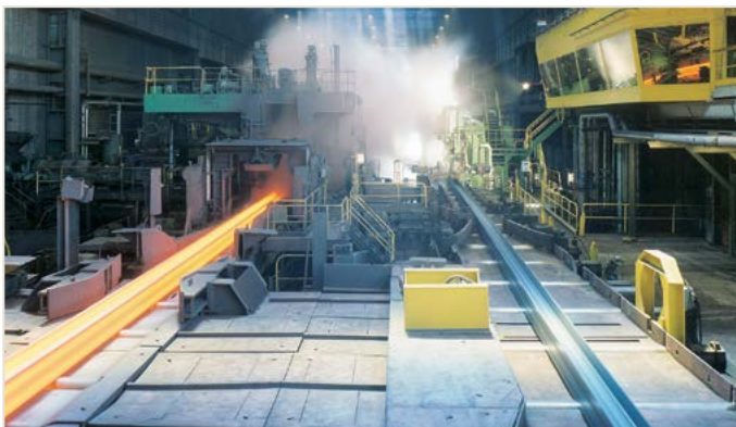
Rolled section entering QST bank (left)
