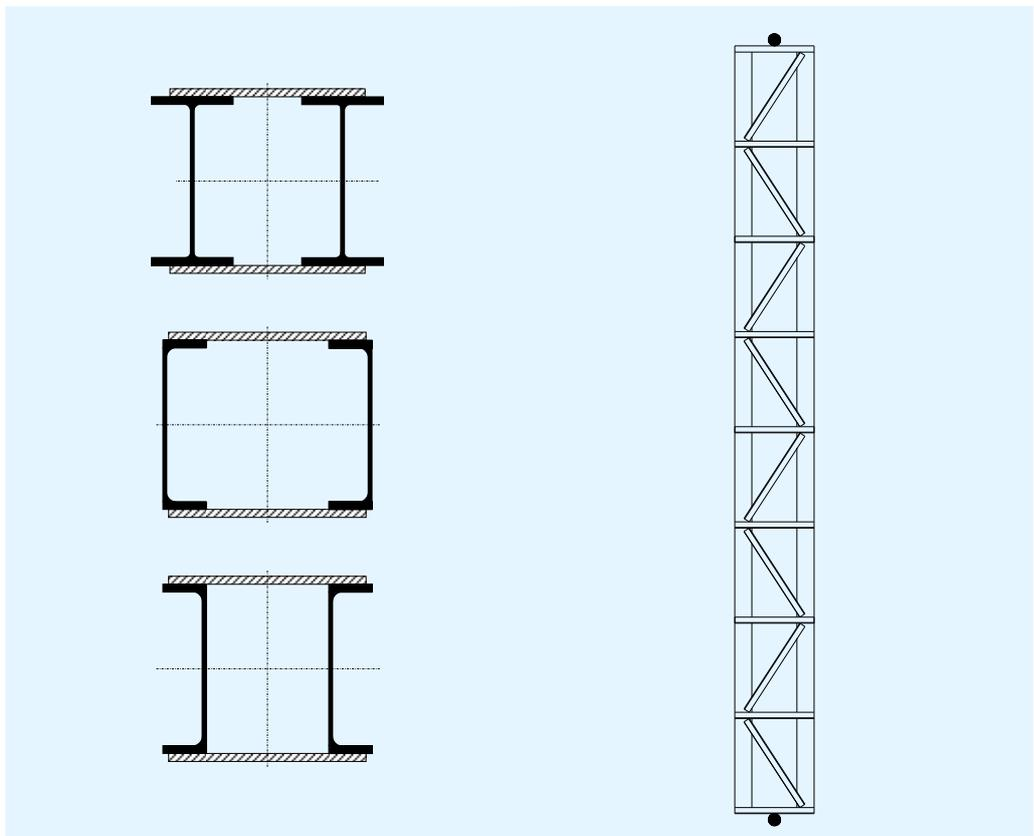
**Figure 2.1 Post for cladding with pinned ends**
