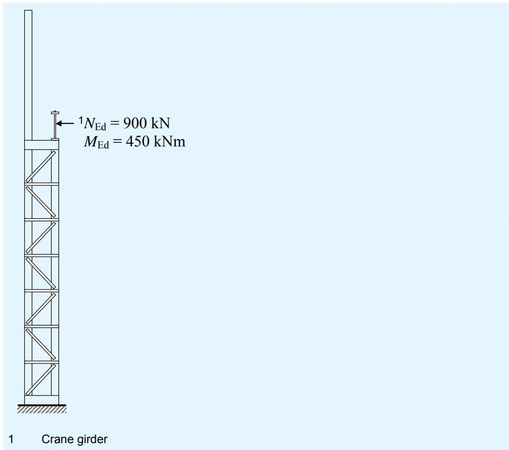
**Figure 2.2 Built-up column supporting a crane girder**
