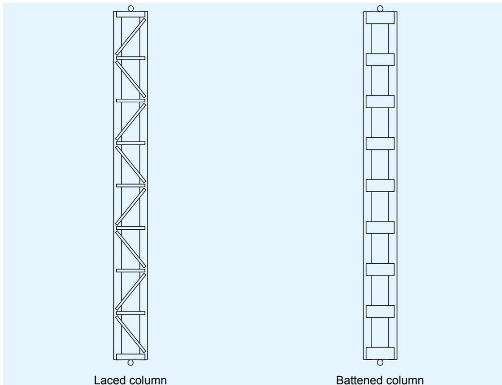
**Figure 2.3 Built-up columns**
