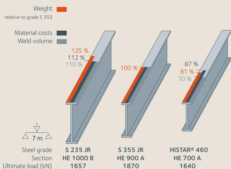
In case of bending, the required cross section and fabrication cost can be reduced by using beams in HISTAR® grades (see Figure 6).
