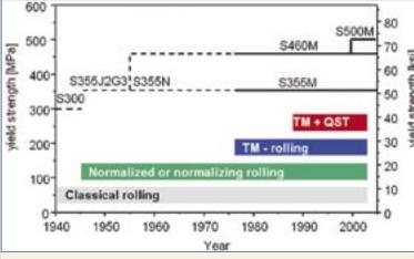
HISTAR 460 (High STrength ARcelorMittal) steels covered by the European standard EN 10025-1 and the American ASTM A 913/ A 913M "Standard Specification for High-Strength Low-Alloy Steel Shapes of Structural Quality, Produced by the Quenching and Self-Tempering Process, (QST)" allow the engineers to use Grades 355 MPa (50 ksi =345MPa ) and 460 MPa (65 ksi = 450 MPa) steels in their design.
