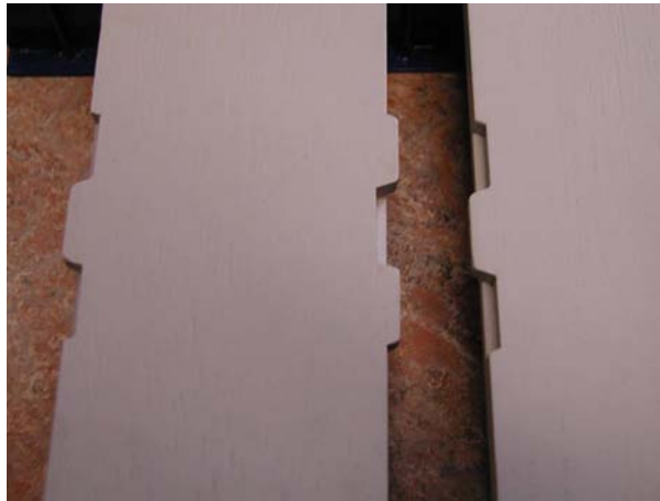
Figure 4-26: Scaled model of fully prefabricated concrete elements, showing the overlapping concrete tongues.
