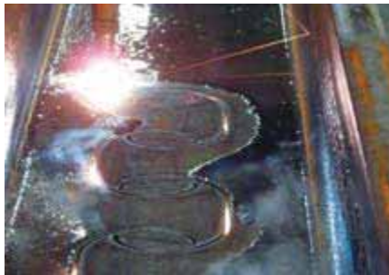
Oxycutting of a rolled beam (HD 320x300 in S460) with MCL shape for a PreCoBeam bridge in Germany.
