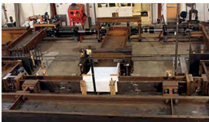
Figure 7.16: Specimen in testing orientation with two actuators.
