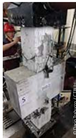
Figure 4.13: Scaled (1:6) Specimen tested to failure
