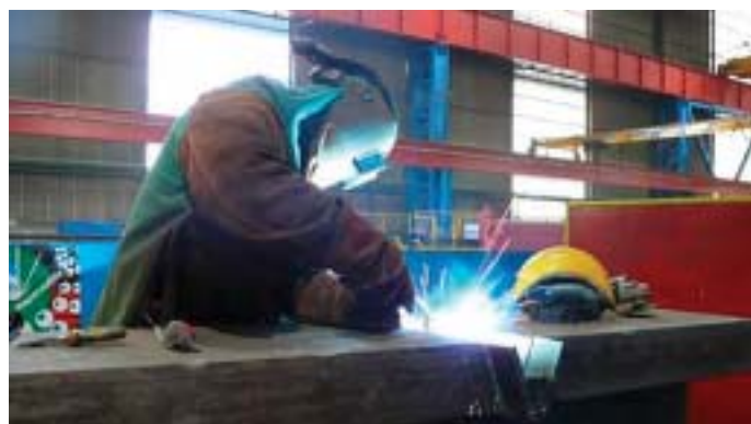
Figure 3.5: Welding of HISTAR® structural steel grades without preheating* (CJP_Complete Joint Penetration_splice of HD400 x 1299 in HISTAR® 460)
