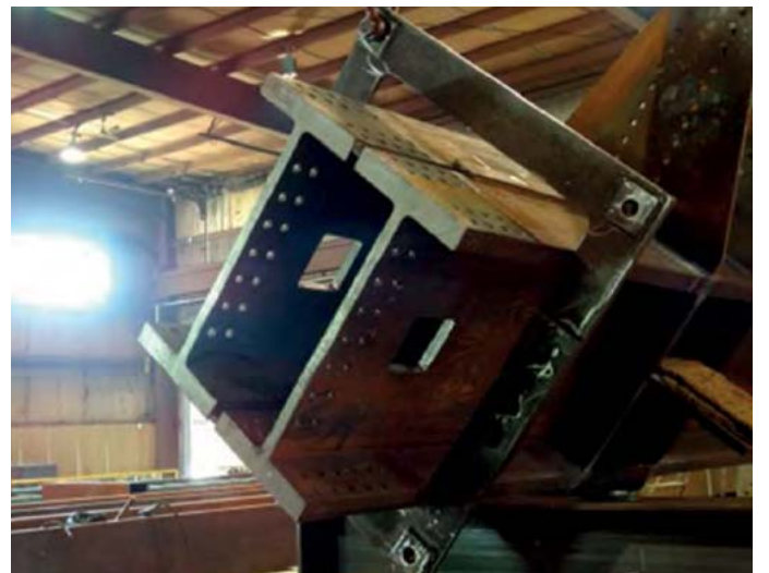
Figure 4.6: Two heavy sections welded together
