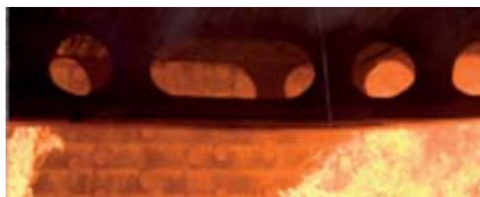
Figure 9.5: Fire test on unprotected cellular beams (FRACOF)
