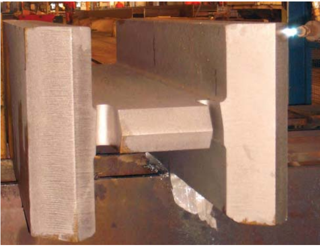
Figure 7.12: Bevel preparation on Jumbo
