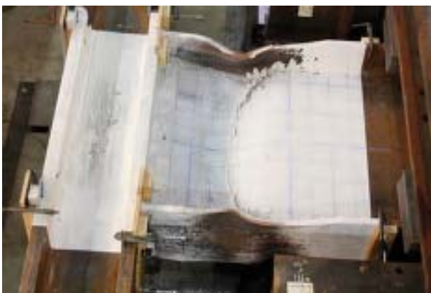
Figure 11.6: RBS: Reduced Beam Section Plasticisation
