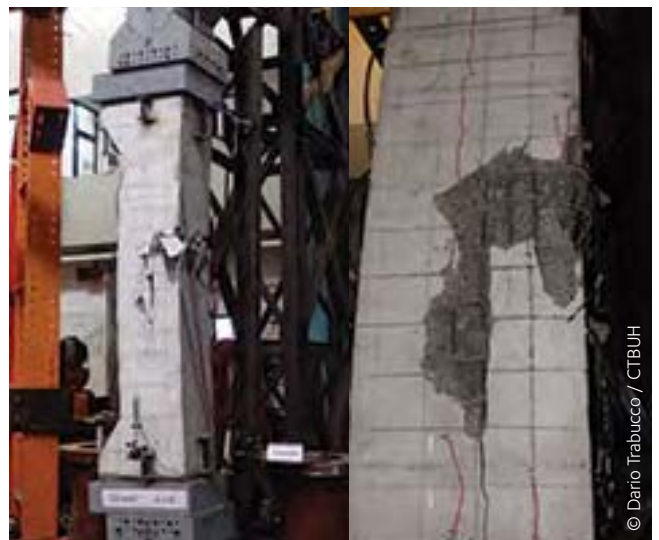
Figure 4.11 Mega-Column scaled (1:4) Specimen tested to failure
