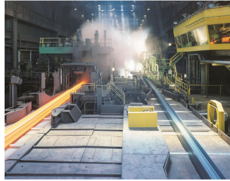
Figure 4: Rolled section entering QST bank (left)
