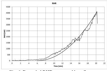
Fig. 6. Recorded RHR curve and best fit curve
