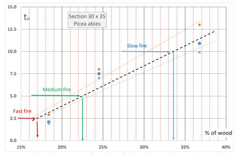
*Fig.* 7. Parameter  $t_{\alpha}$  (in minutes) as a function of the volumetric wood content in the fire load
