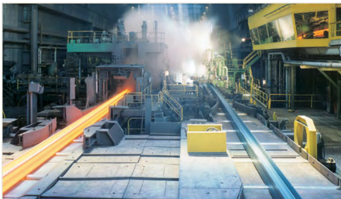
Rolled section entering QST bank (left)
