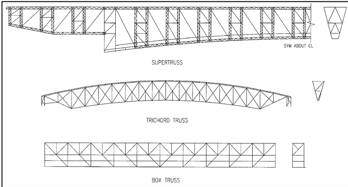
*Figure 3: Reliant Stadium Roof Truss Forms*
