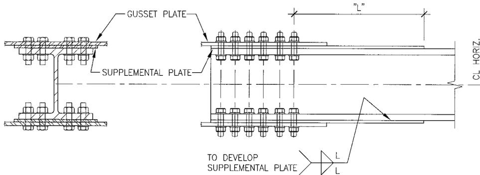
Figure 6: Typical Supplemental Plate Detail
