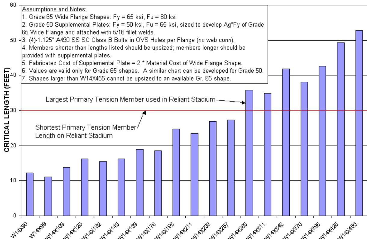
Figure 7: Minimum Lengths for Economical Use of Supplemental Plates for Grade 65 Tension Members
