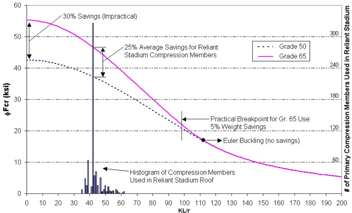
Figure 5: Grade 50 vs. Grade 65 Column Curve
