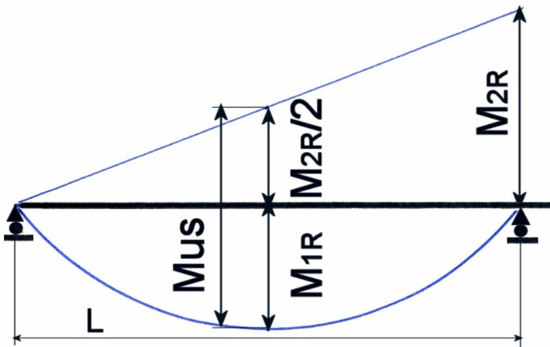
figure 6 – Scheme of the moment redistribution for an edge bay of the continuous beam
