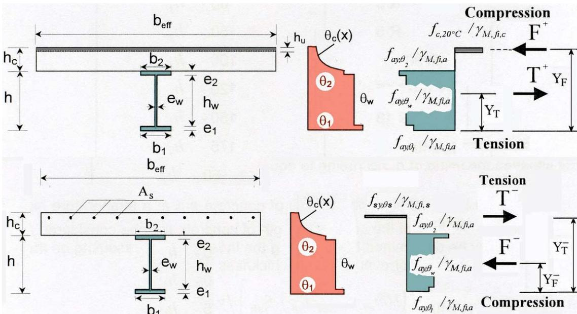
figure 5 – Plastic verification of the composite sections for sagging and hogging moments respectively
