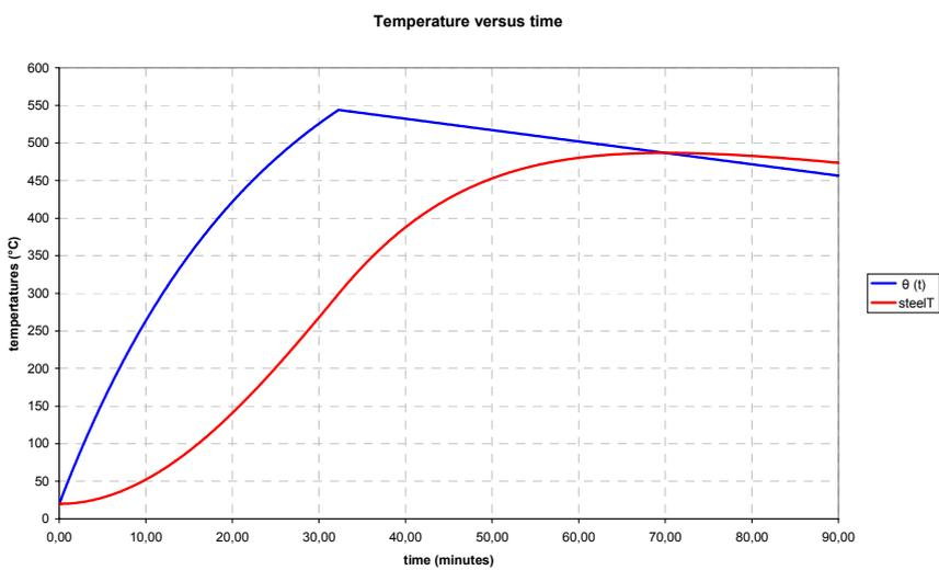
figure 8 - Calculated temperatures at the secondary beam mid span for the ventilation controlled fire
