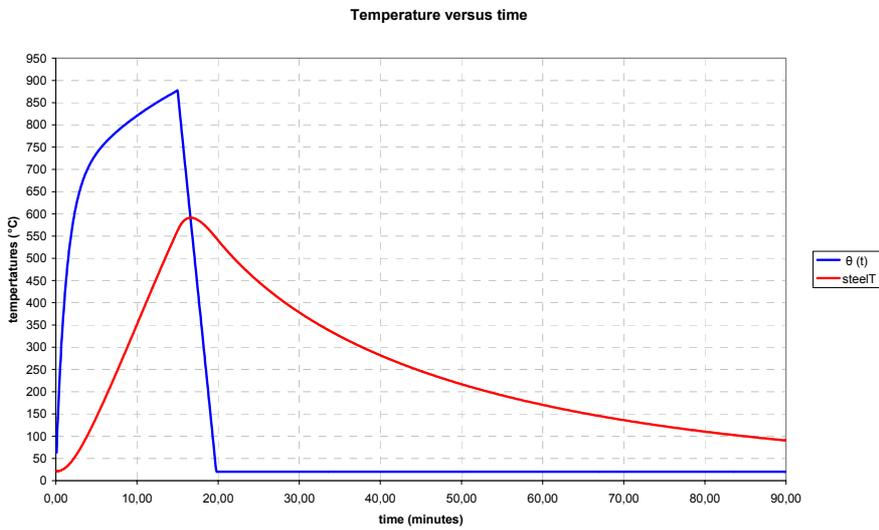
figure 7 - Calculated temperatures at the secondary beam mid span for the fuel controlled fire
