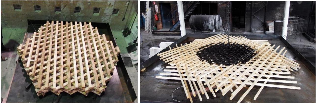
*Fig. 2.* a) Fuel arrangement before the test b) Isotropic horizontal propagation
