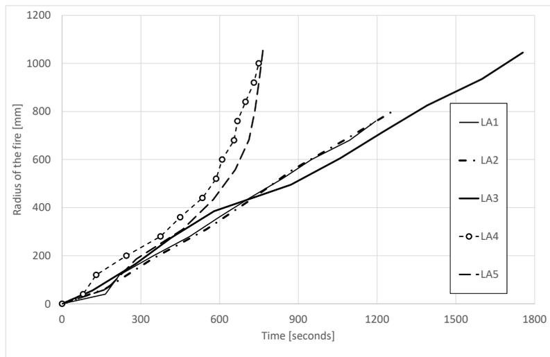
Fig. 3. Evolution of the radius of the fire in the tests LA
