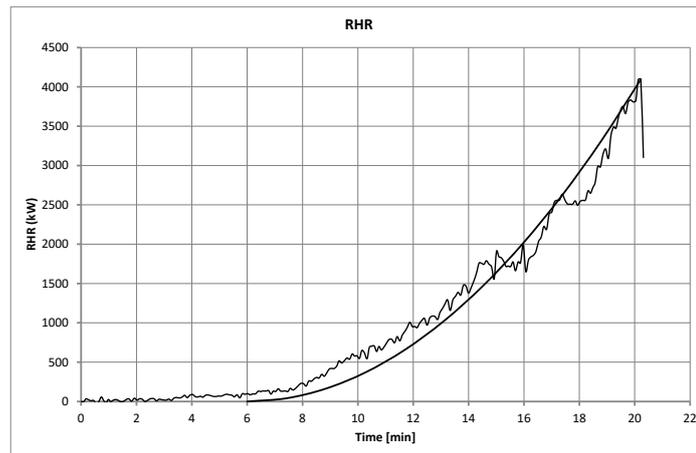
Fig. 6. Recorded RHR curve and best fit curve
